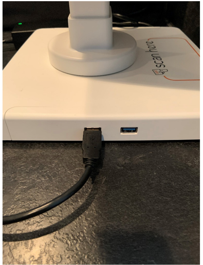
Printer USB Cable Plugged into stand, can be plugged into either port
